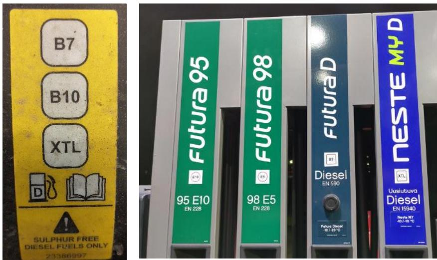
Figure 22: Actual photos of fuel markings (truck fuel tank and fuel dispenser).
